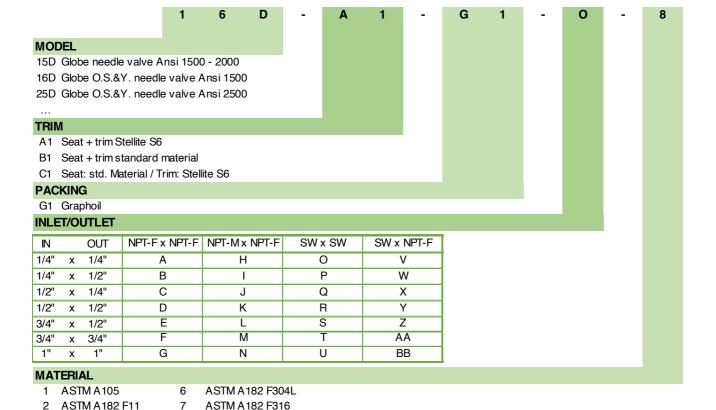
Note: In models 16D and 25D, the material of the components marked with "\*" on the respective example pages does not vary, regardless of the material selected in this table.
