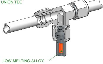
This type of fire sensor doesn't require particular instructions for the assembling :
