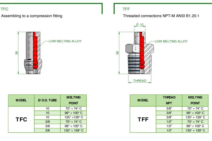
Using the fire sensors we can realise a valid fire detection system, of easy installation, free from any maintenance and of the maximum safety. The fuse element has constituted by a low melting alloy containing bismuth/indio, tin and lead having the following main characteristics.
