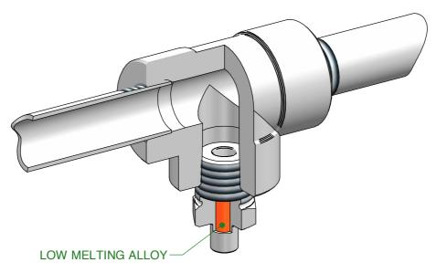
Easier is the assembling of this type of fire sensor, which can be installed in any threaded fittings.
